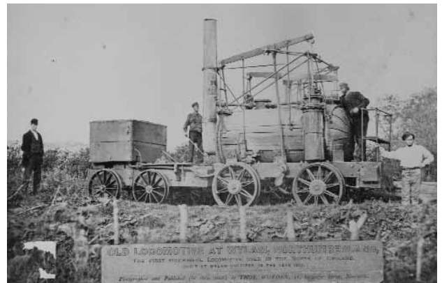
The Puffing Billy locomotive, 1860. This pioneering locomotive was built by William Hedley in 1813 for use on the Wylam Colliery line. The line went from Wylam, Northumberland, to Lemington on the River Tyne. The line had opened in the 1750s, with the wagons being pulled by horses, but Puffing Billy was able to haul much larger loads. The locomotive was used at the colliery until 1860.
